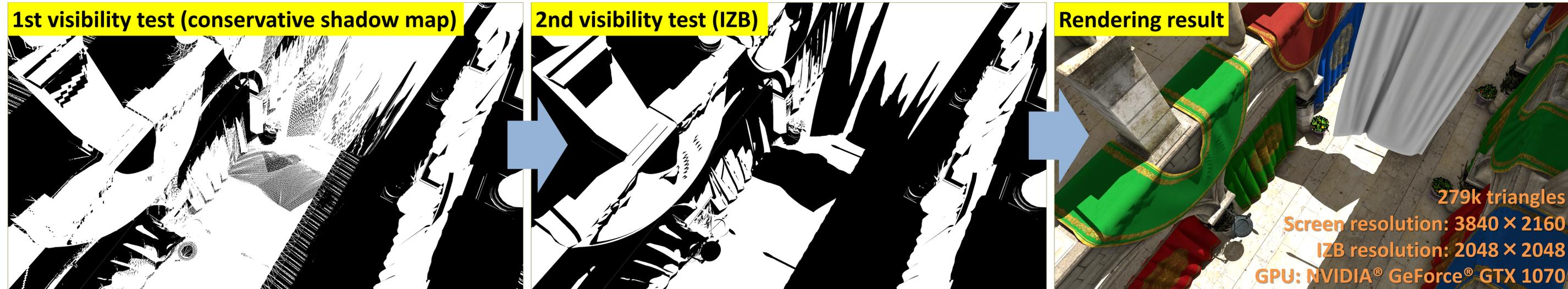
Two-pass visibility test for hard shadows. The visibility is first roughly tested (a) using a conservative shadow map, and then an accurate visibility test using an irregular z-buffer (IZB) is performed only for the remaining shading points (b). Using this pipeline, the shadow performance is **improved from 8.52 ms to 3.59 ms** for the 4K screen resolution.
